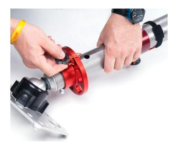
Lock the two elements with the specially provided pin.
