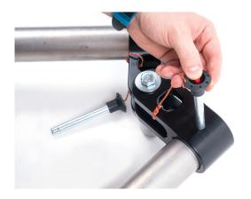
Lock the head on the leg holes and insert the pin.
