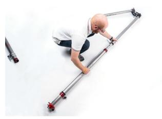
Insert the leg - extractable element - inside the fixed element.
