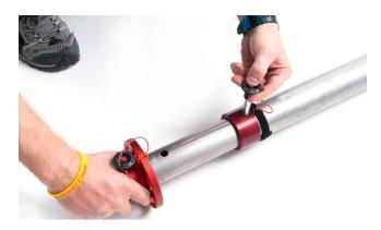
Lock the leg - extractable element - on the hole and insert the locking pin.
