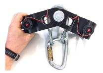
Connect the steel cable loops under the bipod head using an EN362 steel carabiner connector as shown in the figure to the side.
